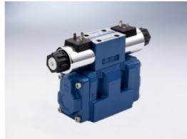
Electro-hydraulic directional control valve is a control valve which can use the pressure of the hydraulic circuit to pull the spool and change the hydraulic oil direction.
